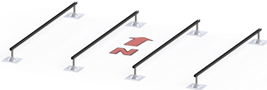
Figure 1.3: Base Strut, Intermediate Framing North-South
